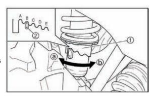
To decrease the spring preload, turn the adjusting ring in direction (b) .
