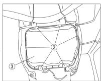
7. Inspect the paper air filter and verify it is okay to reinstall. Softly brush off accumulated dust if necessary. Install a new filter as necessary.
